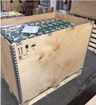
Side walls of NEFAB package is mounted.
