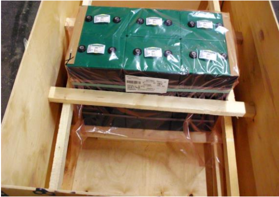
Battery cells are positioned with wooden beams on an EUR-pallet, strapped on top with cardboard in between.
