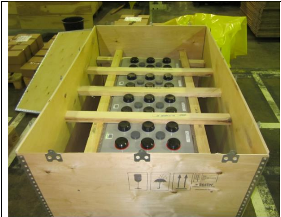
Wooden beams are mounted on top of the battery cells and fixed on the side walls of the NEFAB package.
