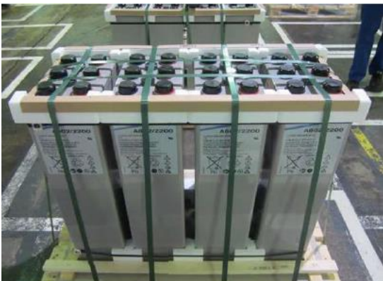
Battery cells fixed with plastic lashing straps and wooden beams on the EUR-pallet.
