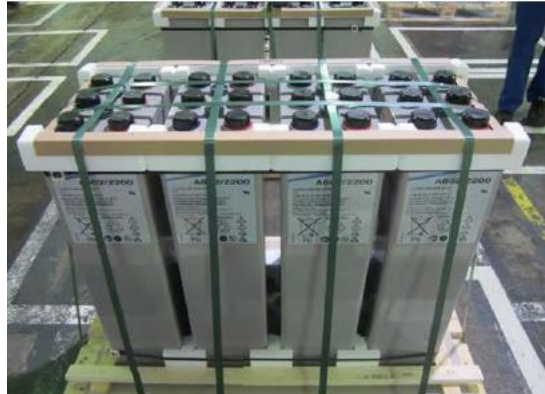
Battery cells fixed with lashing straps and wooden beams on the EUR-pallet.
