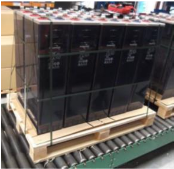
Battery cells are positioned and fixed with cardboard beams and with lashing straps on an EUR-pallet.
