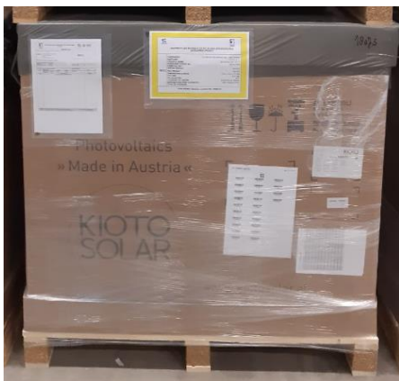
Cardboard with PV modules, labelled and marked. The cardboard box is on top covered with an oversized PE foil, to avoid ingress of water, wrapped with foil and finally secured with plastic lashing straps.
