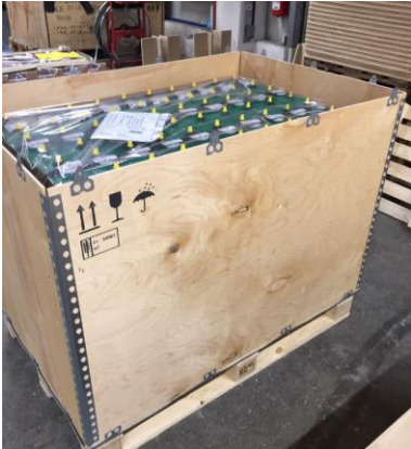
Side walls of NEFAB package is mounted.
