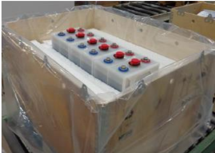
A strong plastic bag is placed in the NEFAB box. The battery cells with polystyrene plates are placed in this bag to fix it correctly.
